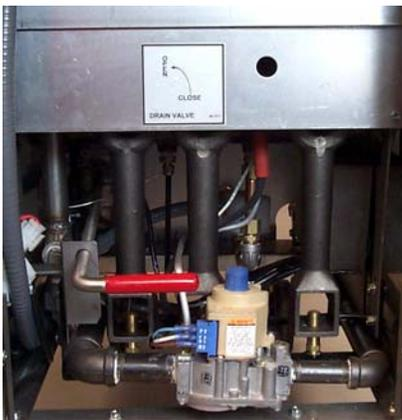
Gas valve and drain handle on spark-module equipped unit.
